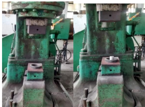
Figure 5: Ring stopper and loading of work piece
